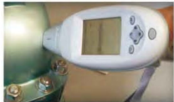
Spectrograph( For testing of chemical composition analysis)
